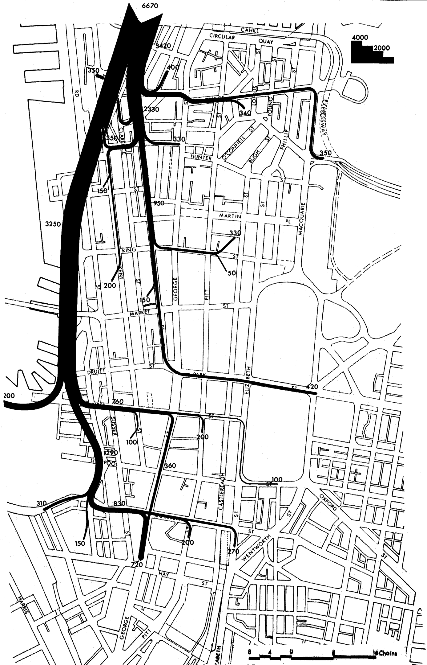
Fig. 9 Year 1970 – Simulated Distribution of Southbound Traffic from Sydney Harbour Bridge during Morning Peak Hour on Basis of Western Distributor Stage I and Northwestern Expressway having been Completed. (Vehicles per Hour)
